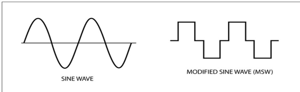
If you want to run your equipment exactly to the manufacturer's specifications, choose a pure sine wave inverter. With pure sine wave, motor loads start easier and run cooler. Some equipment only operate properly with pure sine wave inverter, such as laser printers, variable speed motors and digital clocks.
